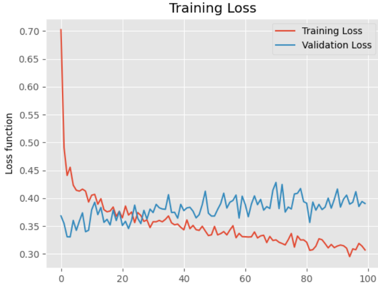
Figure 5.2: An (unrelated) example of clear overfitting, the validation loss increasing after some time
