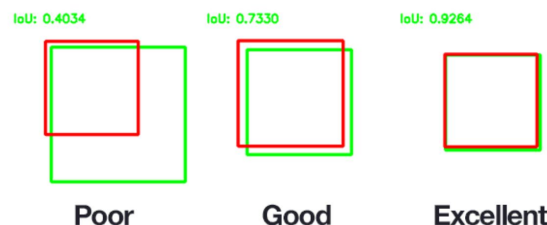
Figure 2.23: Illustration of the value of the Intersection over Union score according to the positions of the bounding boxes, the red one being the ground truth bounding box and the green the predicted bounding box. © [50]
