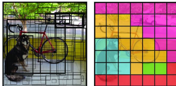
Figure 2.20: On the left image: bounding boxes and their confidence score, where the higher the confidence score is, the thicker the boundaries of the box are. On the right image: the class probability map, where the blue cells indicate that the class "dog" is the most probable one, the yellow cells correspond to the class "bicycle", the pink cells to the class "car" and the red cells to the class "dinning table". © [46]
