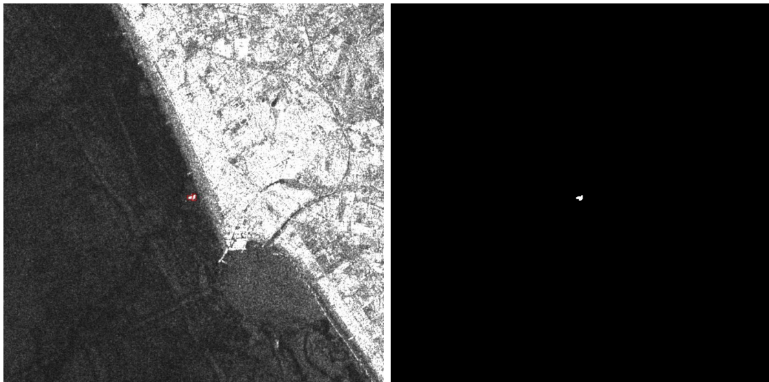
Figure 6.6: Image 02_6_28.jpg and its mask. Two detections are against each other and are not distinguishable to the human eye. The corresponding masks are joined.
