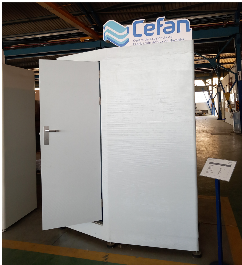
Figure 45: Cefan: 3D printed bathroom
