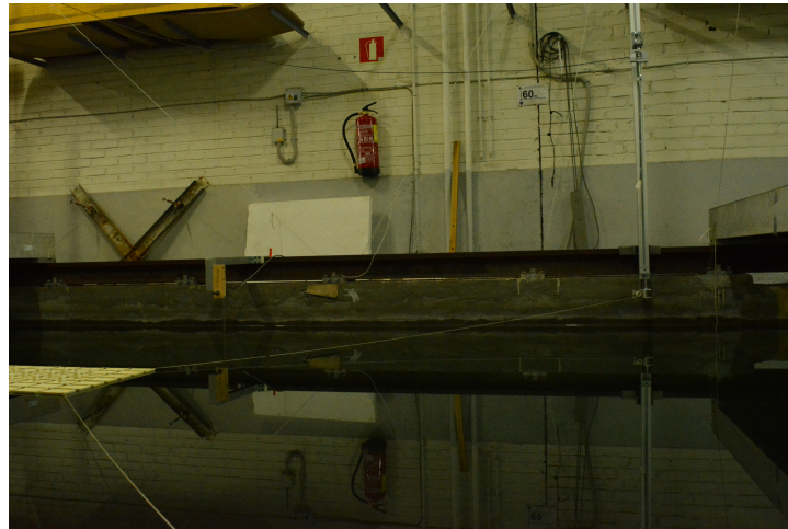
Figure 28: Parabolic shape of mooring line in 1:60 scale model.
