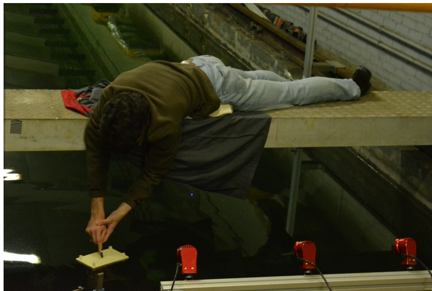
Figure 29: Execution of a decay test on a single panel.
