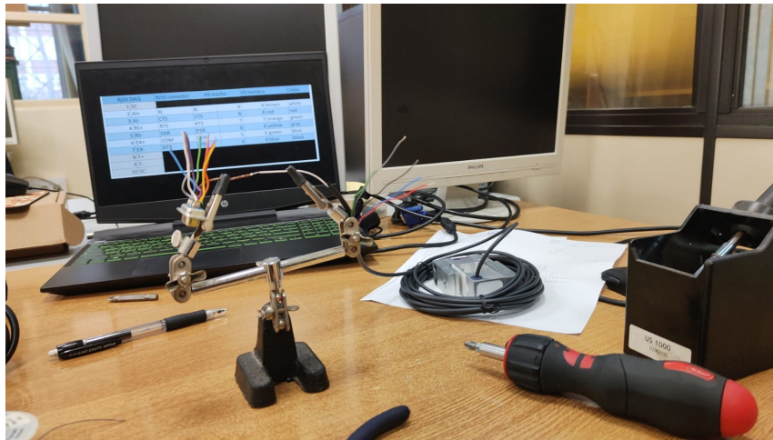
Figure 21: Welding of a load cell to a RS 232 connector.
