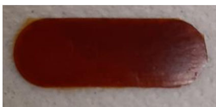
Fig. 26: Liquid bis-cyclic carbonate and TREN-based implant
