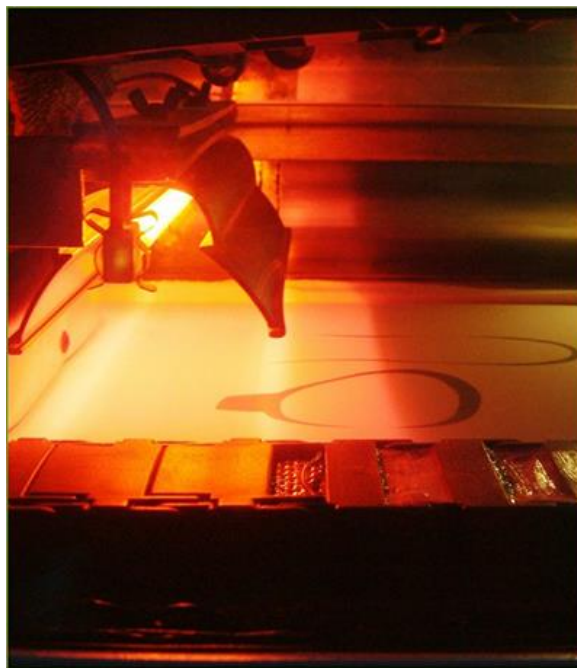
(16) Illustration du processus de production additive PBF
