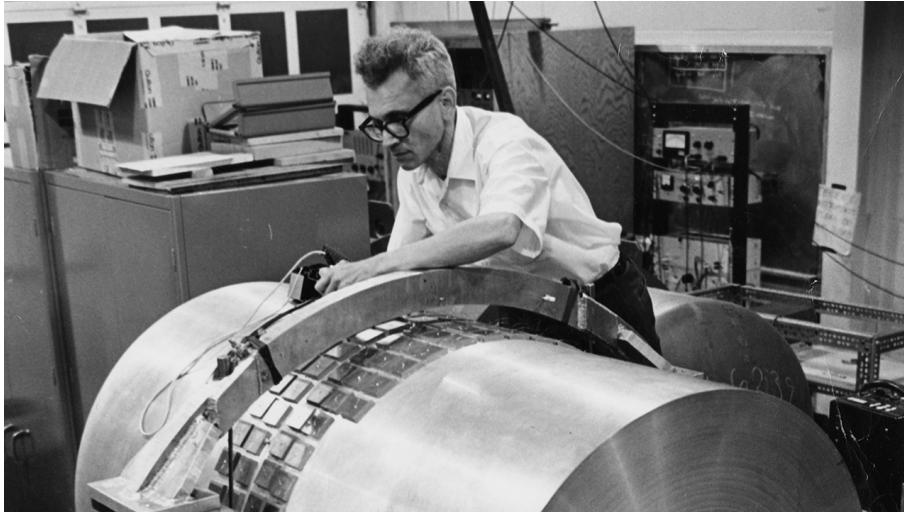
Figure 1.2: Joseph Weber besides one of his gravitational wave detector bars, at the University of Maryland [5].
