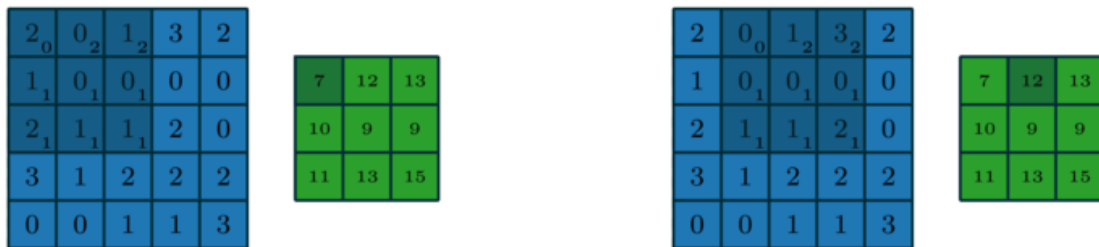
Figure 2.7: An illustration of the convolution operation of an input of size 5x5 by a kernel of size 3x3, with a stride of 1. Figures adapted from [37] using [38].
