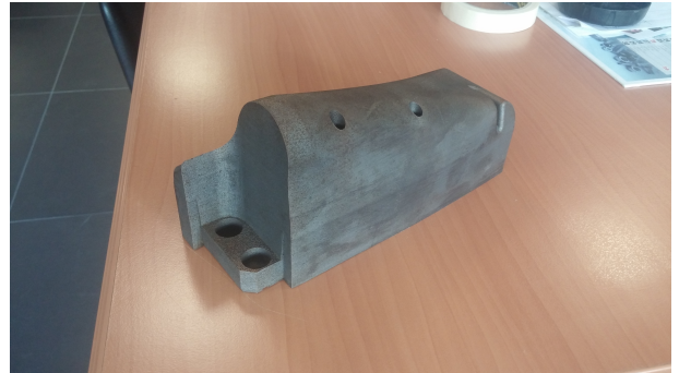
FIGURE 3.2: Part obtain by reverse engineering and 3D printing
