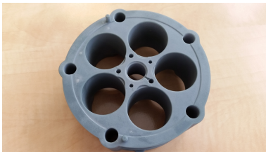
FIGURE 3.3: Compressor print in accura bluestone, it is a high mechanical property polymer
