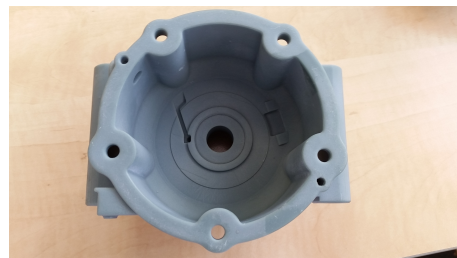
FIGURE 3.4: Compressor print in accura bluestone, it is a high mechanical property polymer
