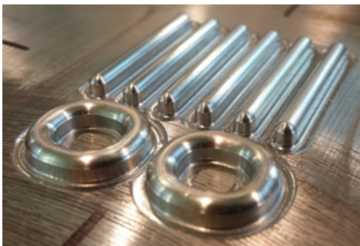
FIGURE 6.16: Die manufactured by DED, machined finish
