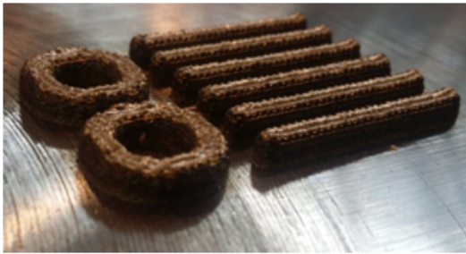
FIGURE 6.14: Die manufactured by DED, raw finish
