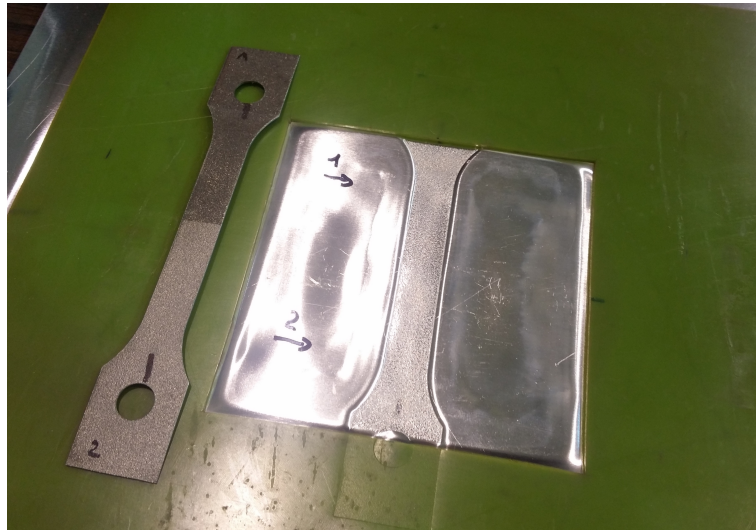
FIGURE 6.13: Test 1: Reproduction of surface quality; 1050, 11.5 kJ
