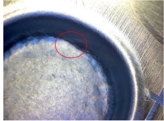
FIGURE 6.30: Test 2: Crack on the bottom of pocket
