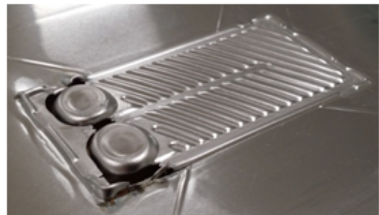
FIGURE 6.24: Test 9: Machined die; Al 3003 at 8.8 kJ, gap 1.3
