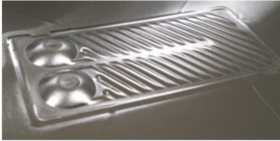
FIGURE 6.21: Test 6: Machined die; Al 3003 at 4 kJ, gap 0.3
