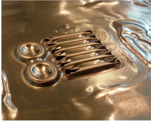
FIGURE 6.18: Test 4: DED die and machined finish; Al 3003 at 8.8 kJ
