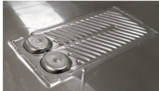
FIGURE 6.22: Test 7: Machined die; Al 3003 at 11.5 kJ, gap 0.3
