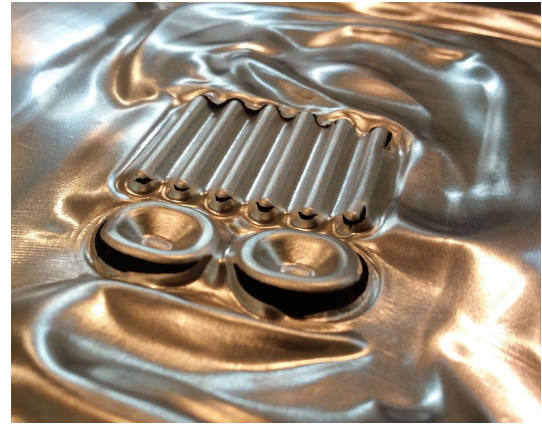
FIGURE 6.19: Test 5: DED die and machined finish; Al 3003 at 4.5 kJ, gap 2 mm
