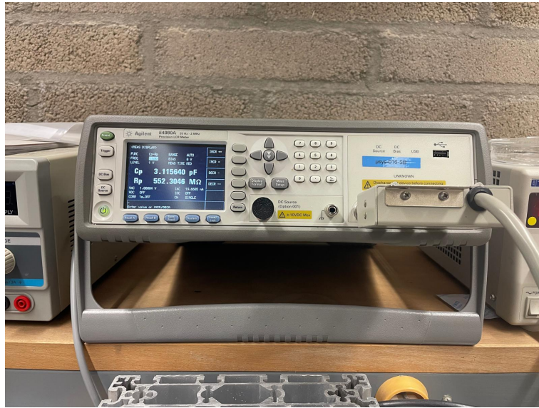
Figure 3.16: LCR Meter used for capacitance measurement
