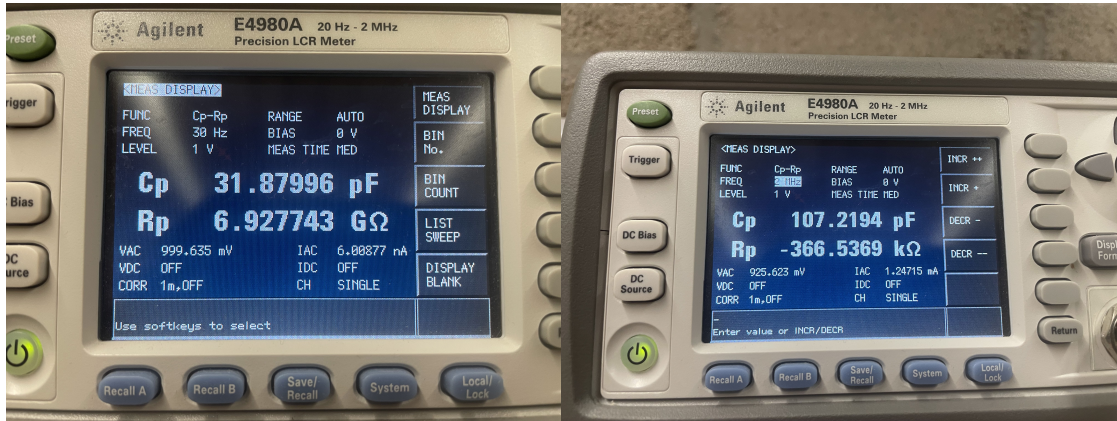
Figure 4.6: Minimum Capacitance value obtained at maximum plate distance Figure 4.7: Maximum Capacitance value obtained at initial charging
