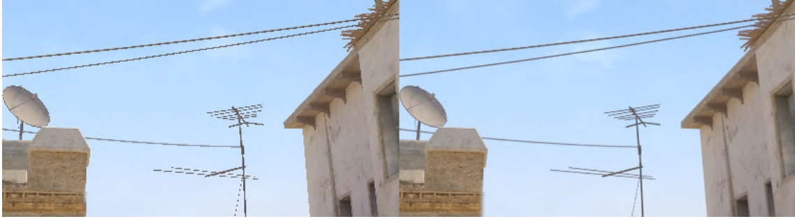
Fig. 2.5: This figure shows a comparison between a render with and without anti-aliasing. Some aliasing artifacts are visible on the left image, whereas on the right image, those aliasing artifacts are less pronounced at the cost of image sharpness. Both images were rendered at a 1920x1080 resolution, the left render did not have any anti-aliasing method enabled whereas the right render had 8x multi sampling anti-aliasing enabled. Both images are taken from the game Counter-Strike 2 at the exact same position.
