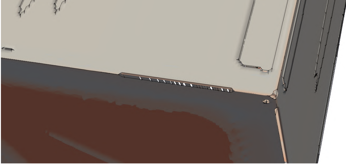
Fig. 5.11: This figure shows an example of the output of the Flying Edges algorithm without the smoothing step. The output presents holes and black artifacts.
