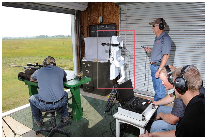
Figure 2.5: Experimental setup featuring a shooter, Doppler radar system, and the Hornady 3 engineering team conducting ballistic coefficient measurements [54].
