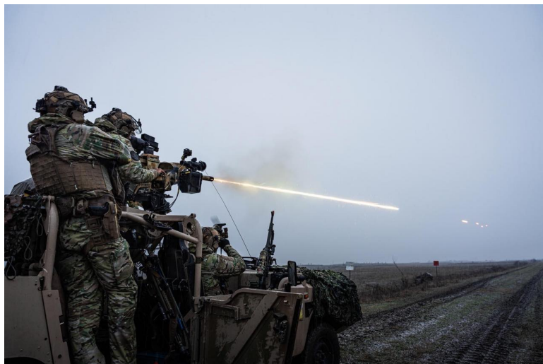
Figure 1.3: Rapid Reaction Vehicle crews (RRV) of the Belgian 2 nd battalion commando [102] equipped with GMG [61] chambered with tracers. This type of projectile is built with a small pyrotechnic charge in its base. When fired, it emits visible light, aiding shooters in tracking their trajectory and making real-time adjustments (especially in low-light conditions).
