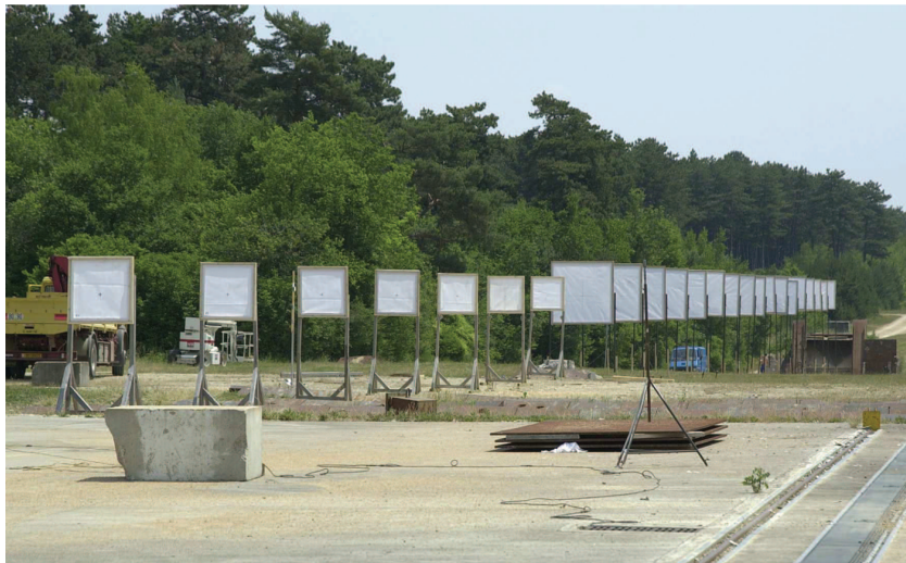
Figure 2.6: Yaw cards at the DGA Tt shooting range in Bourges (FRA) during tests for Nexter Munitions 4 [36].
