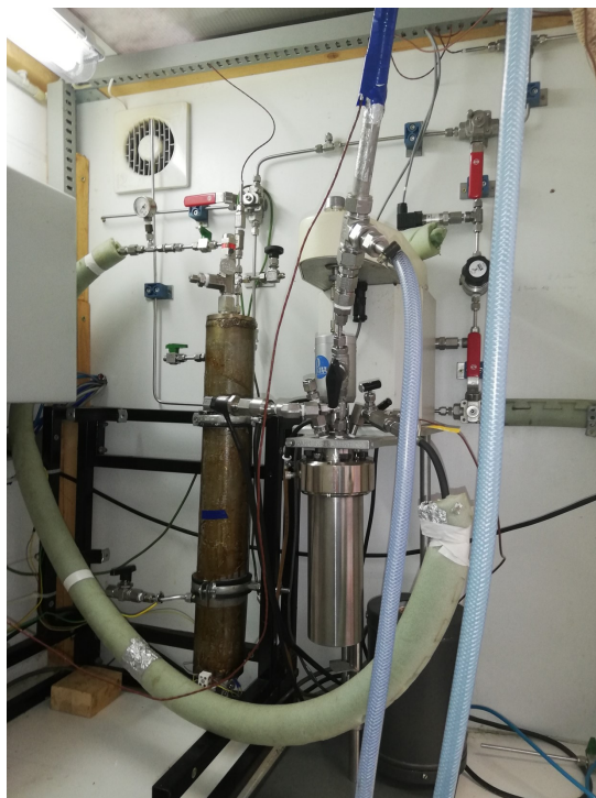
Figure II.13: Degradation reactor and water balance control parts
