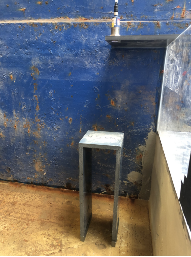
FIGURE 2.19: Photo of a shim under the sensor for calibration purposes
