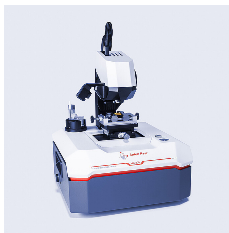
(b). Picture of nanoindentation tester, used for real testing at nanoscale [64].
