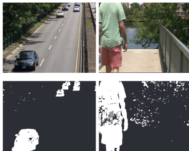
Figure 1.2. Example of a foreground extraction. The top image is the original frame, the bottom image is the foreground mask. The white pixels represent the foreground, and the black pixels represent the background. Source: [6].
