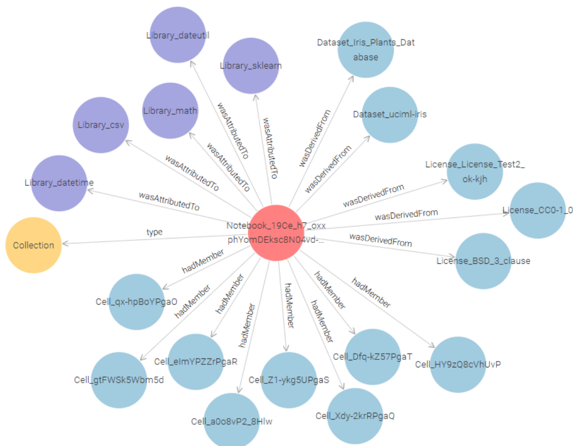
Figure 6.1: Visualization of a notebook and its properties in the knowledge graph with GraphDB. The notebook is of type Collection and is represented with its cells, libraries ( datetime , math , etc.), datasets, and licenses.
