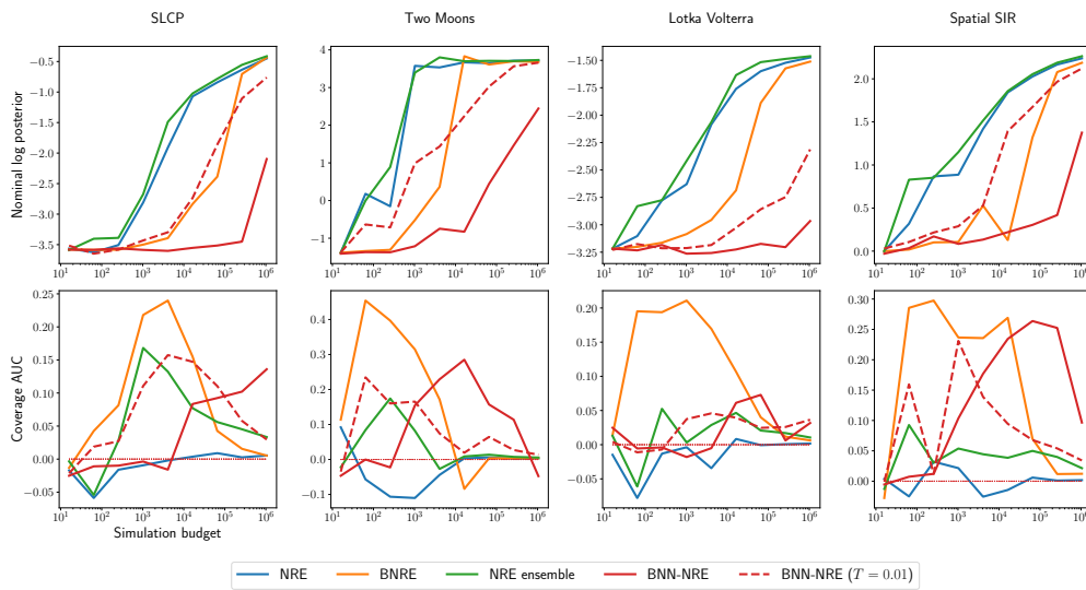
Figure 7: Comparison of different NRE simulation-based inference methods through the nominal log probability and coverage area under the curve. The higher the nominal log probability, the more performant the method is. A calibrated posterior approximation exhibits a coverage AUC of 0. A positive coverage AUC indicates conservatism, and a negative coverage AUC indicates overconfidence. 3 runs are performed, and the median is reported
