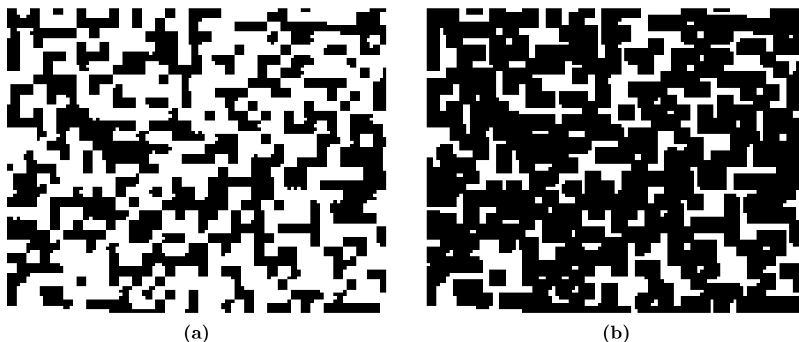
Figure 4.13: Comparison between the pattern mask before and after morphological erosion. (a) Zoomed-in view at the center of the pattern mask before erosion. (b) Same portion of the pattern mask after the morphological erosion.
