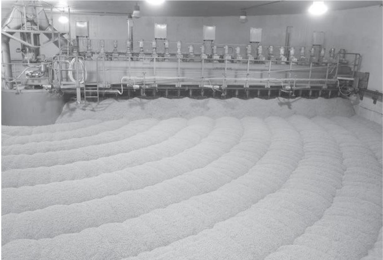
*Fig. 4.1: This Circular germination bed is 92' (28 m) across and 63" (1.6 m) deep. It holds 400 metric tons of barley per batch; the harvest from about 200 acres of local farmland.*
