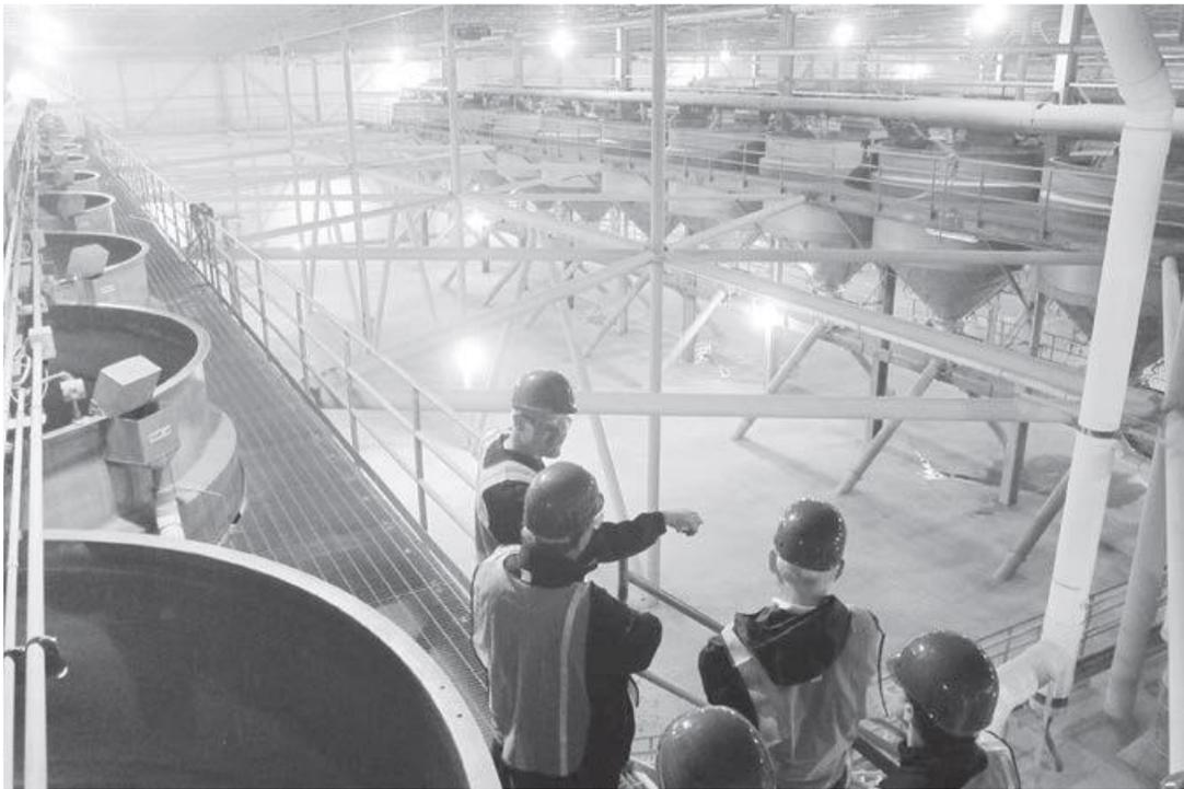
*Fig. 4.3: Steep tanks at a modern malthouse. 12 tanks are used for each 200 metric ton (441,000 lb) batch of malt. Salad box germination beds are located directly below the steep tanks.*
