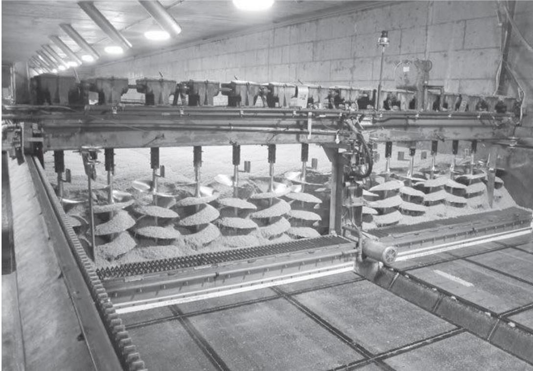
*Fig. 4.6: Saladin Box-type germination bed in the process of being “stripped” to the kiln.*
