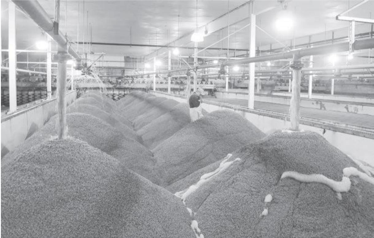
*Fig. 4.2: Loading the Saladin boxes with grain from the steep tanks. The barley is moved as a slurry and its distribution in the bed is manually controlled at this malthouse.*
