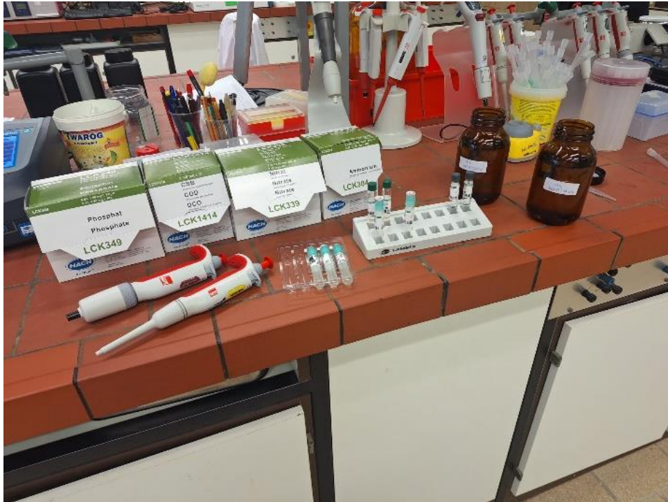
Figure 7: Hach tests for COD, NO 3 , NH 4 , PO 4 measurements
