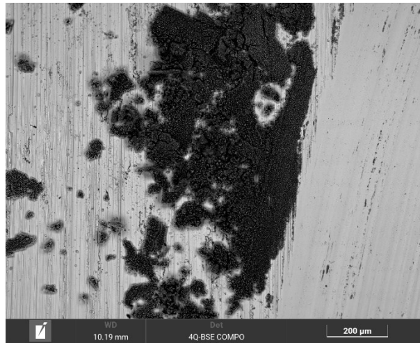
Figure 54: Crushed debris of the RT1500 wear test. The micrograph is taken in the same position as Figure 52.c one.
