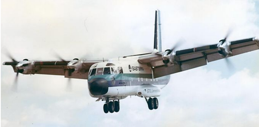
Figure 2.2.1: Breguet 941 during approach with inboard/outboard flap deflected at 98^\circ/65^\circ , source unknown.
