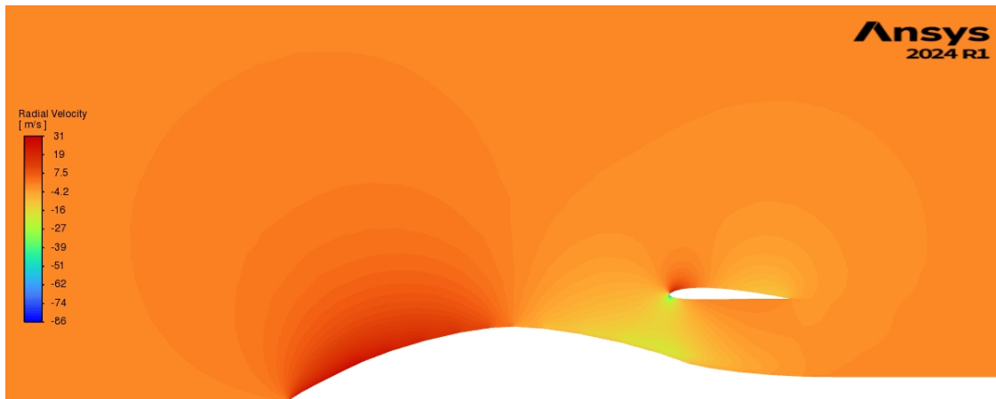
Figure 3.13 - Radial velocity (along y) in axisymmetric and cruise conditions.
