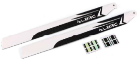
Figure A.3: Blade ALZRC 325 mm [5] and closest airfoil shape Eppler E171 [7].
