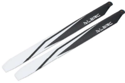
Figure A.4: Blade ALZRC 380 mm [4] and closest airfoil shape St. CYR 172 [10].
