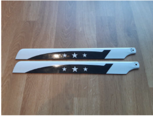
Figure A.2: Blade BL450 325 mm [31] and closest airfoil shape Göttingen GOE 411 [8].
