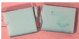
Figure 2.28 – Sample 2 with c/t = 0.05 after fracture.
