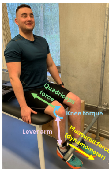
Figure 2.4: Illustration of the forces and moments acting on the knee during a quadriceps contraction measured by a dynamometer.
