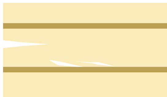
Figure 1.12: Illustration of the crack propagation in transversal loading of the cortical bone.
