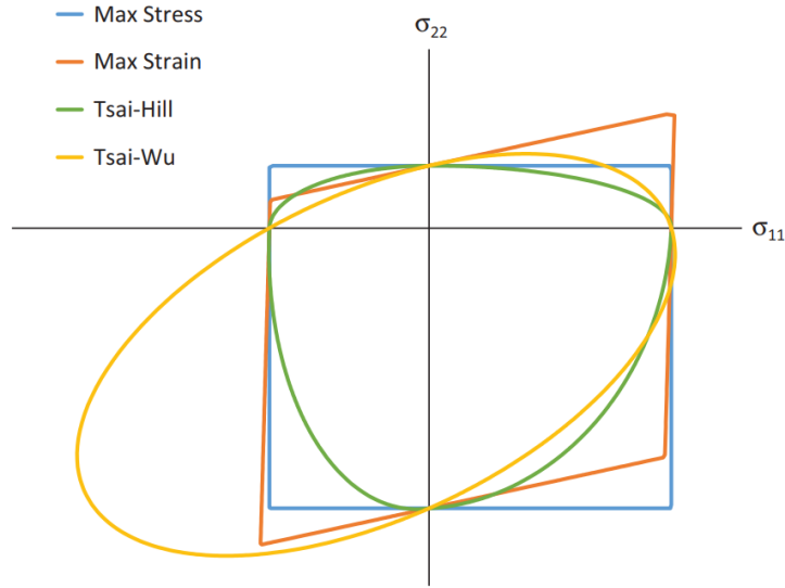
Figure 2.12: Comparison of the different failure envelopes defined by the failure criteria. From [31].
