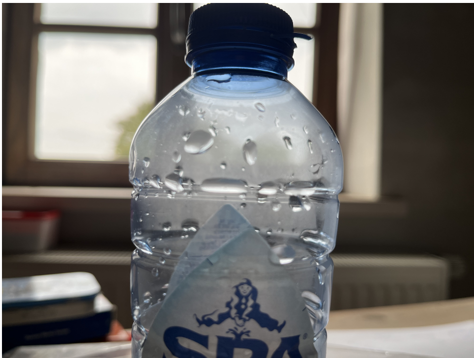
Figure IV.1: Near the neck of a water bottle, some droplets remain at their position without moving, despite gravity trying to drag them down. This is an effect of contact angle hysteresis.
