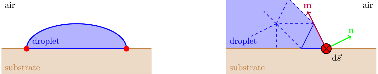
Figure III.3: Representation of the boundary \partial\Gamma_L \equiv \partial\Gamma (red dots) and its tangent vector d\mathbf{s} (noted d\vec{s} in the figure) as well as the vector \mathbf{m} . The figure on the right is a zoom on the right side of the droplet.
