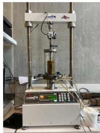
FIGURE 4.17 – Appareil triaxial
