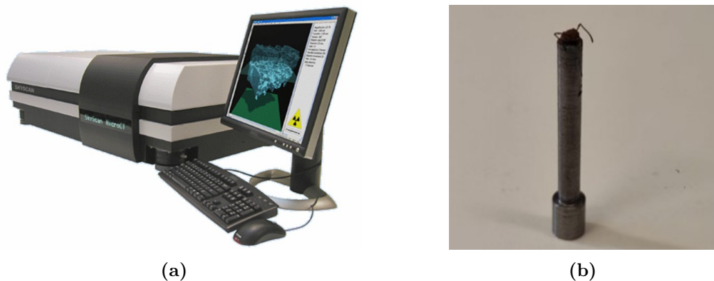
Figure 18: Overview of the microCT scan, Figure 18a from [9] shows the system and Figure 18b showing the sample holder used.
