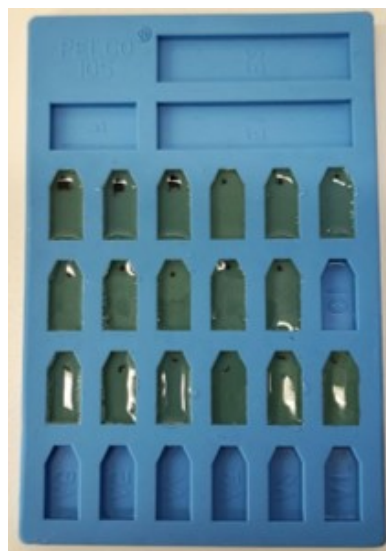
Figure 14: Samples embedded in epoxy resin and oriented inside the molds.
