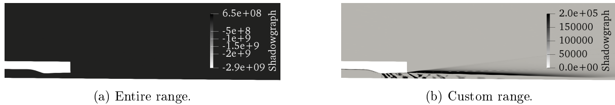
Figure 4.10: Supersonic jet in hot atmosphere: Shadowgraph at the nozzle exit.
