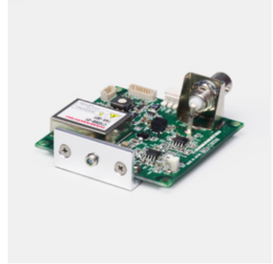
Figure 1.20: Picture of an APD control circuit from Hamamatsu with the the high voltage unit on the left of the picture. Taken from [47]
