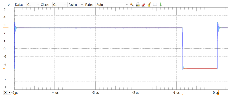
Figure 3.14: Eye diagram of the comparator signal with the emitter and receiver at a distance of 4.5m and with symbol 8 transmitted
