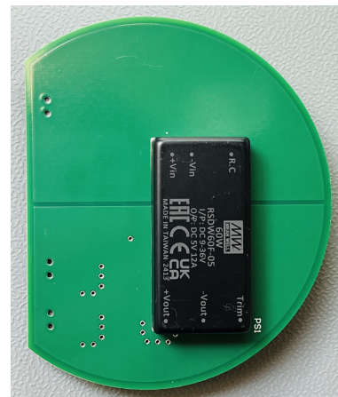
Figure 2.93: Picture of the emitter supply board with its components placed on it (bottom)
