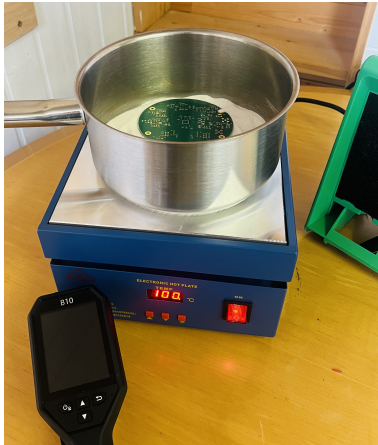
Figure 2.61: Picture of the implemented alternative reflow system.
