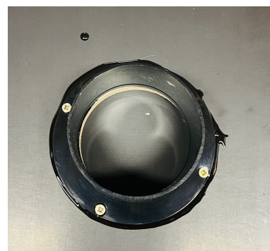
Figure 3.3: Test bench pipe's support glued
