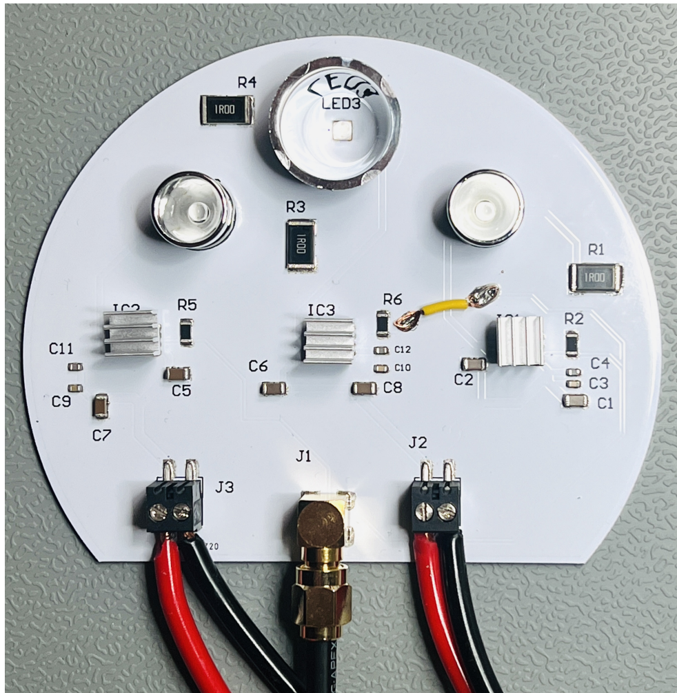
Figure 2.89: Final assembled UWOCS emitter board with their optical concentrators
