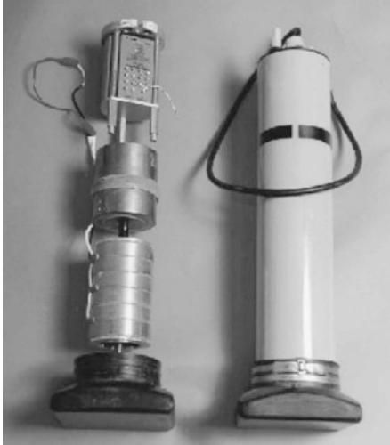
Figure 3: Picture of a Tonpiz acoustic transducer with its piezo stack. Taken from [12] p.10
