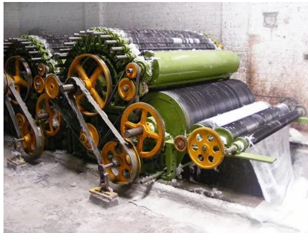
Figure 19. Garnett textile recycling machine (Source: https://www.indiamart.com/proddetail/garnett-machine-14013596412.html )
