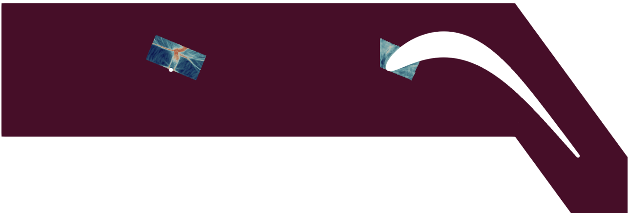
Figure 5.19: AV box around the shock region. Highlight on the domain specification problem.
