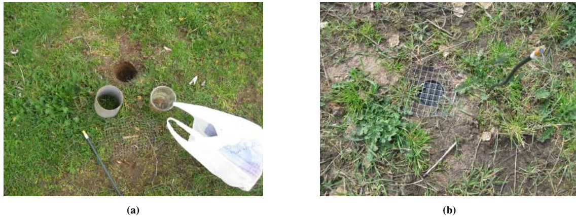
Figure 4.2: Typical pitfall assembly. (a) The PVC plastic piece fixes the hole and holds the glass jar filled with a preservative to collect terrestrial invertebrates. The mesh prevents bycatches and the stick helps to locate the trap. (b) The trap is left for a year, buried up to the rim.
