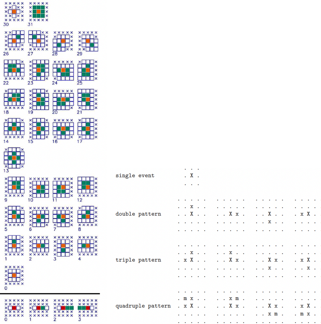
FIGURE 2.9: Left: pattern code of the MOS instruments. The orange boxes represent the main pixel that received the highest pulse impulse (PI), the green boxes are pixels with a PI higher than the detection threshold.
