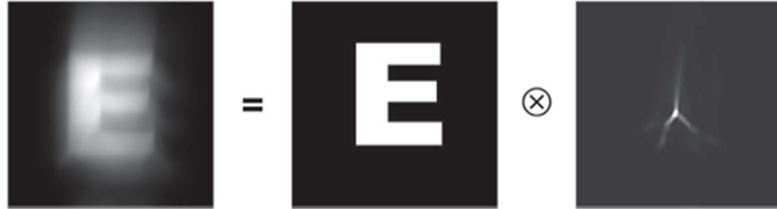
Figure 2.9: Blurred image resulting from the convolution of an original scene with a PSF. From [13].
