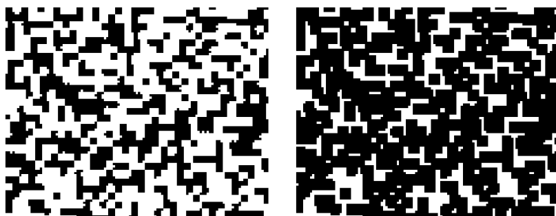
Figure 3.3: Comparison between non-eroded (on the left) and eroded (on the right) patterns for a same mask portion. From [17].
