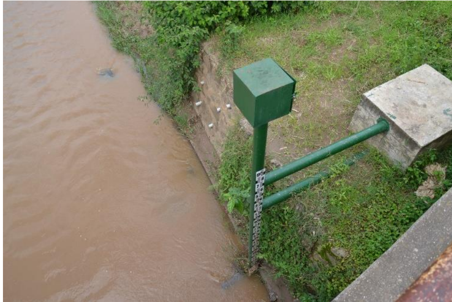
Figure 25. Picture of the Nyarutovu hydrometric station where the Diver is placed. Note the staff gauge attached to the monitoring well (Picture by Victor De Clerck, 2023).
