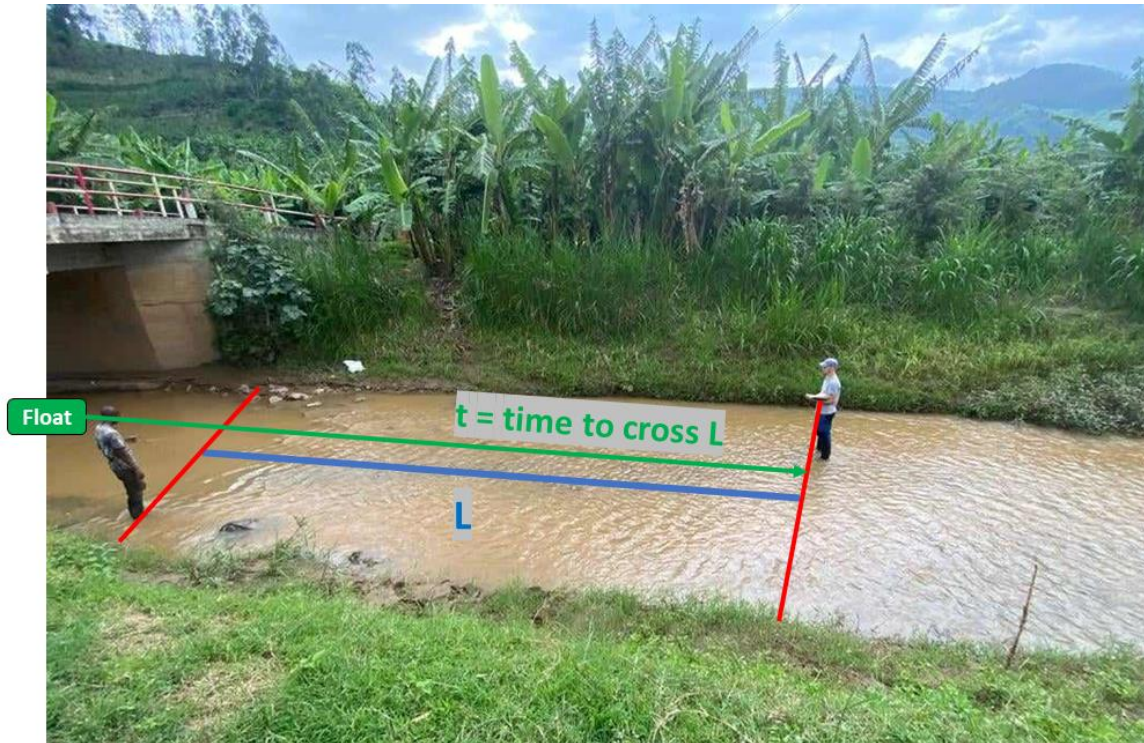
Figure 28. Diagram illustrating the float method for measuring discharge (Picture by Déogratias Nahayo, 2023).
