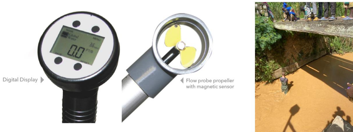
Figure 26. From left to right: 1) pictures of the FP211 flow probe with its digital display, 2) the propeller component (YSI, 2020), and 3) a picture demonstrating the utilization of the FP211 in a river within the Mukungwa watershed (Picture by Déogratias Nahayo, 2023)
