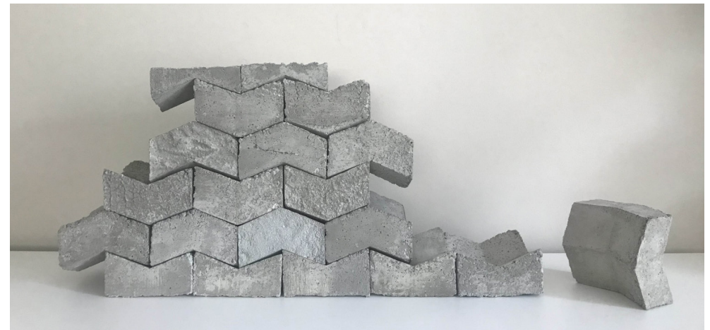
Figure 18: Image showing on of the block prototype made by Yenice, Y., & Park, D. (2019b, January 1). V-INCA - designing a smart geometric configuration for dry masonry wall. eCAADe Proceedings. https://doi.org/10.52842/conf.ecaade.2019.2.515
