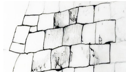
Figure 16: Sketch from based on the Edojou Tenshudai fort in Tokyo to illustrate the process of laying the walls “Kirikomihagi”. [Original drawing©]
