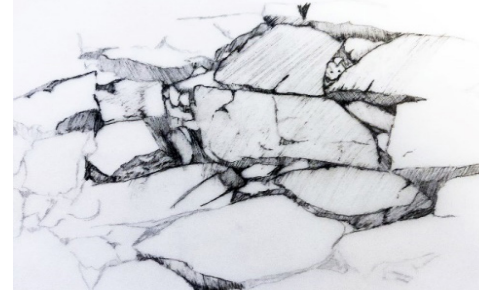
Figure 12: Sketch illustrating the so-called «Ransekiizumi» process used for the Matsumotojou fort in Nagano. [Original Drawing©].
