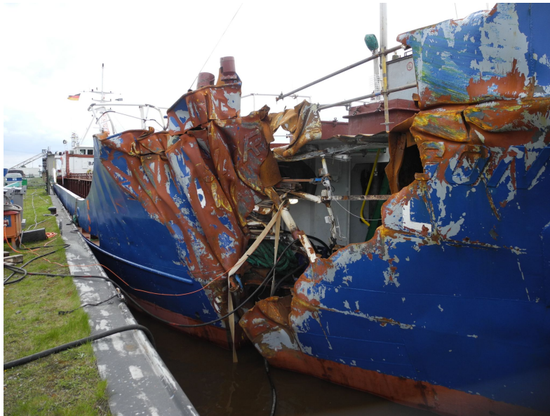
Figure 1: Damaged hull of Petra L after collision with a wind turbine; Source : Buljan (2023)
