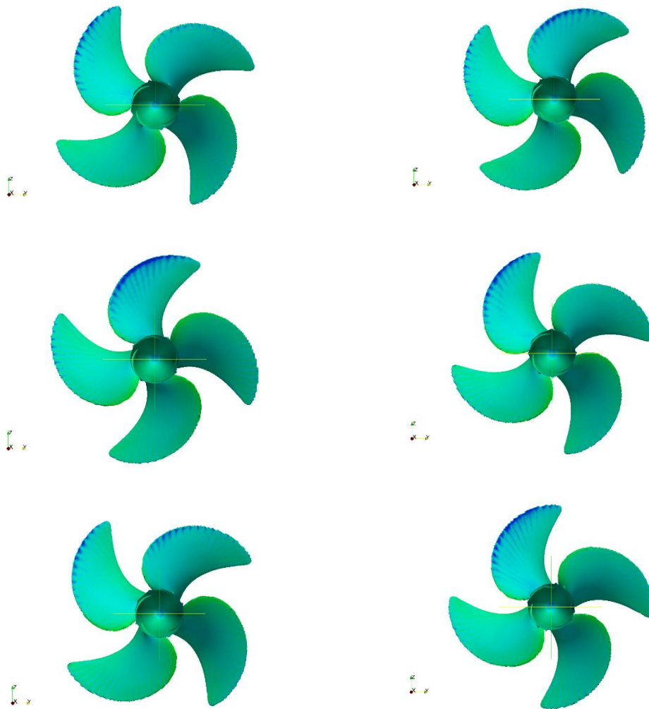
Figure 57. Evolution of the Pressure Field in the Suction Side: High-Skew Angle Blade Profile
