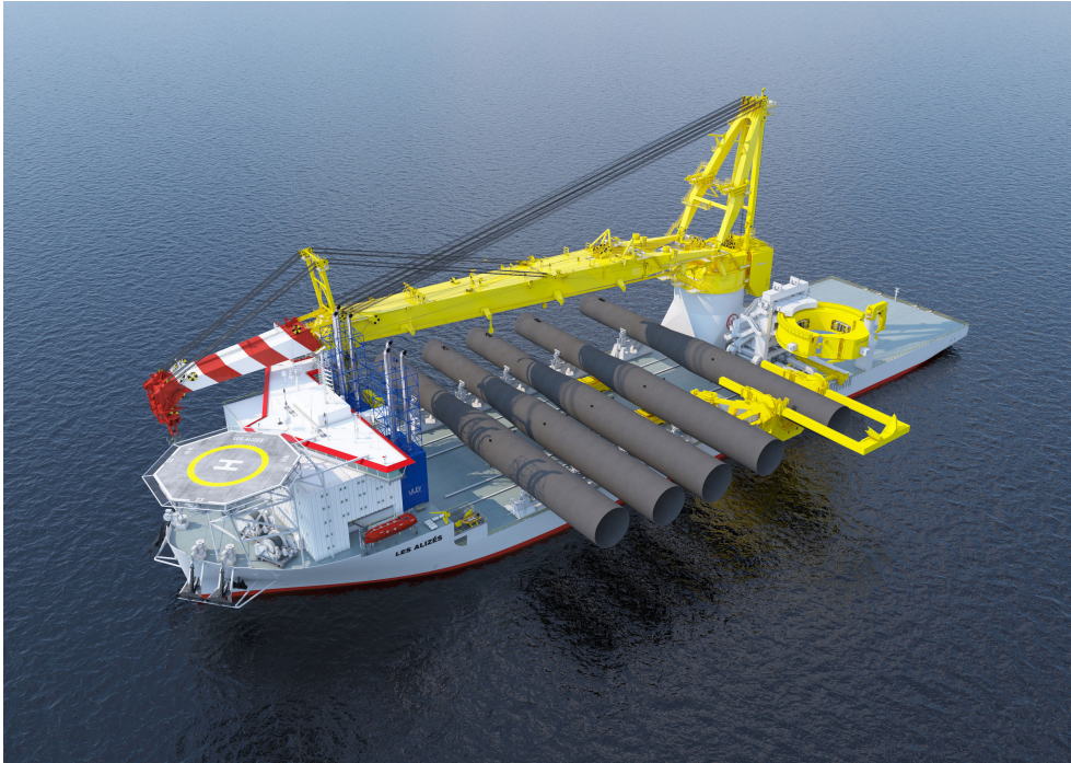
Figure 4.3: Les Alizes loaded with monopiles
