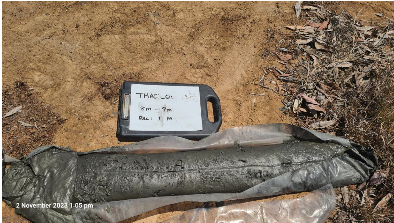
Figure 59: A retrieved sonic drill core.
