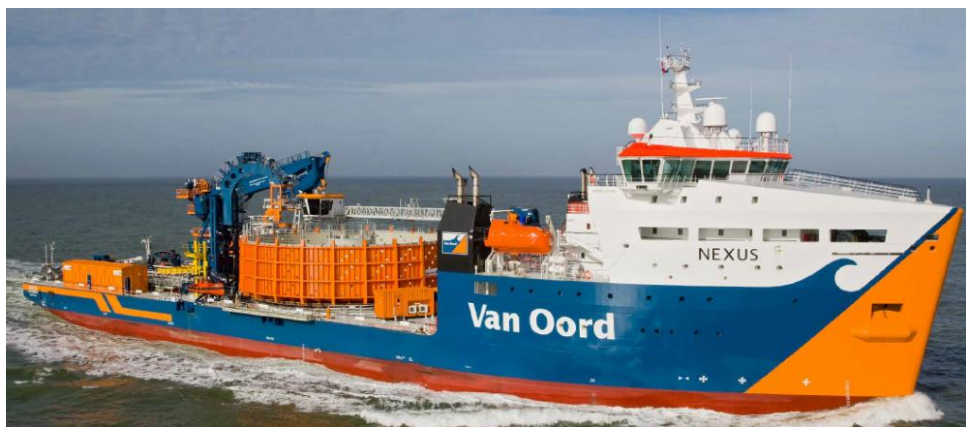
Figure 8: Cable installation vessel [25].
