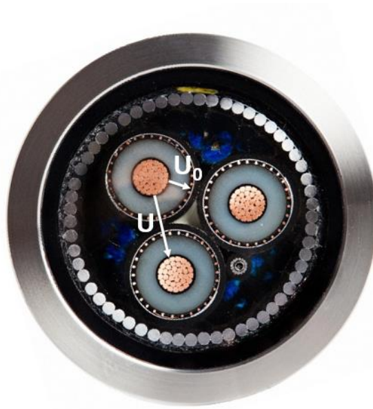
Figure 6: Power cable cross section [15].
