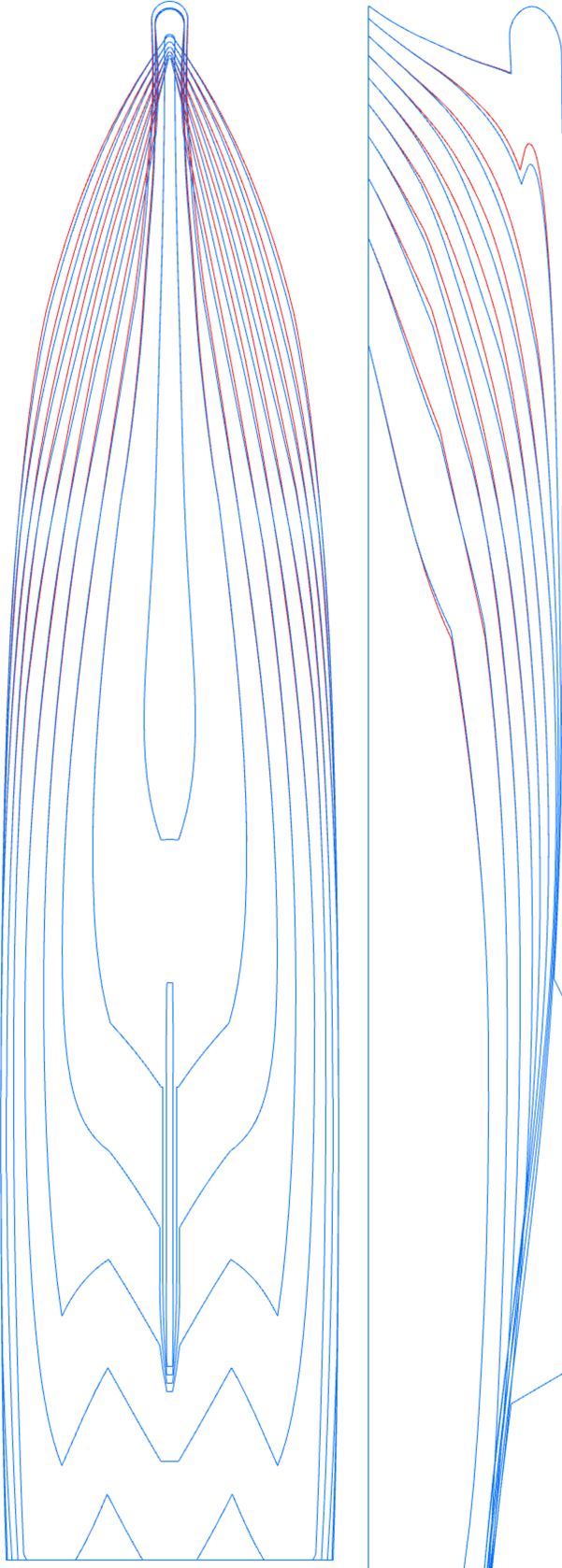
Patrol Vessel Hull Lines (INITIAL & MODIFIED)
