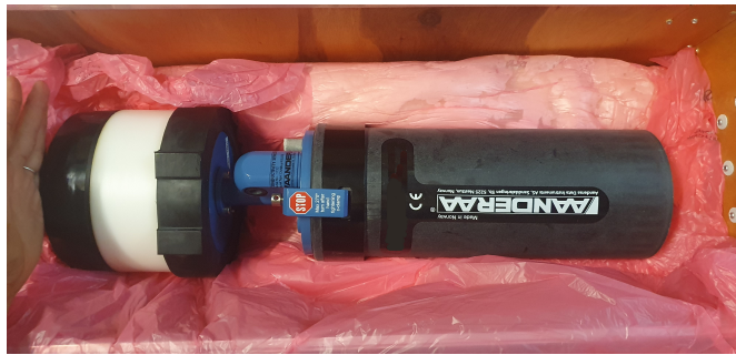
Figure 4: The ADCPs used during the study: Seaguard type II from Aanderaa.
