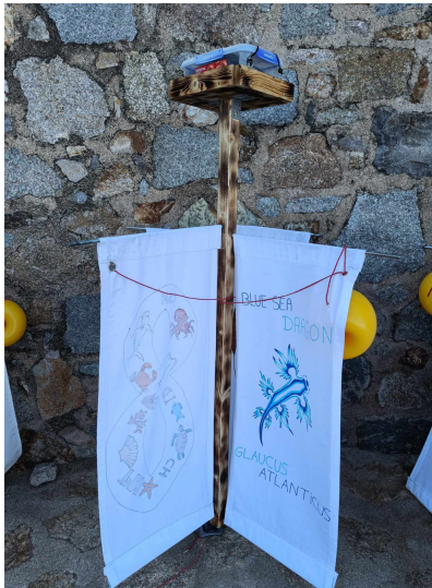
Figure 36: One of the 2024 drifters, made by the Liège oceanography master students and used to measure surface currents in the Bay of Calvi.
