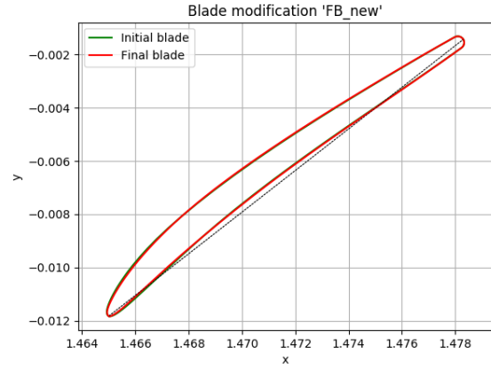
(b) FB comparison with +10% Thickness Shift
