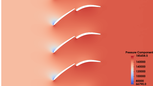
(e) Baseline at inlet flow angle of 56°
