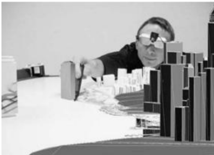
Figure 10 - An augmented user is dragging a model from the toolbox into the mixed real and virtual model space.
